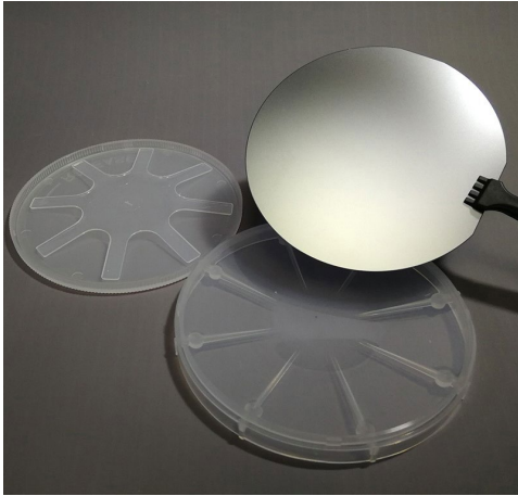
Bulk InSb: Commercial (MTI), (100) orientation, undoped, n-type, rough back side
